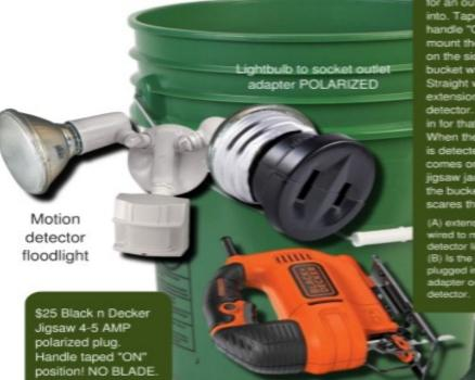
The jigsaw goes in the bucket and you swap one of the light sockets for an outlet to plug it into. Tape the saw handle "ON" and then ount the light fixture on the side of the bucket with bol aight wire the nsion cord to the detector. Leave a bulb in for that surprise too. in the an is detected the light es on and the w jacks around in bucket which es the critter off.
