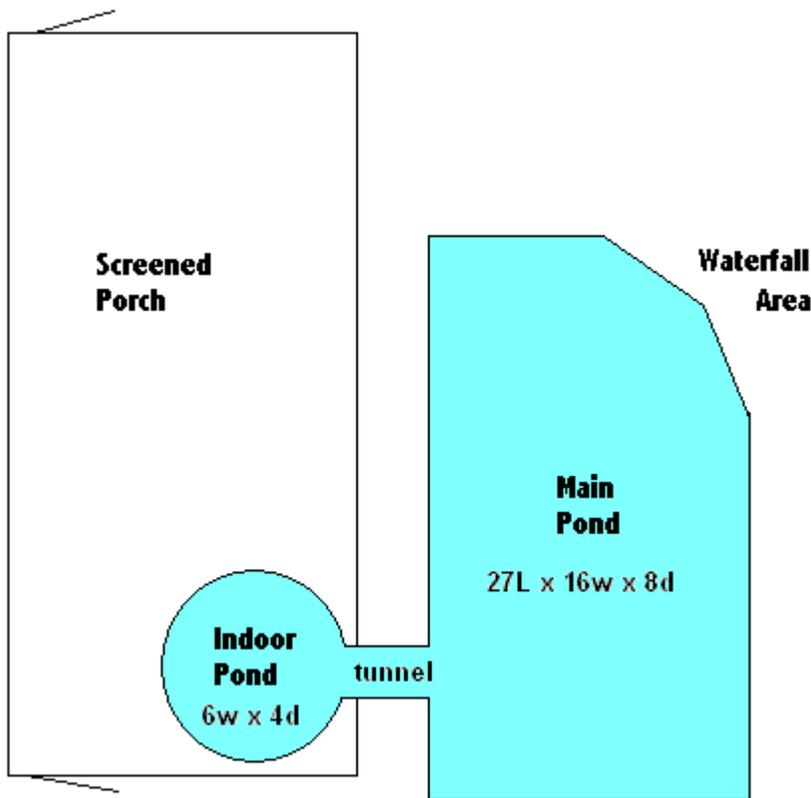
One of the more unique aspects of this pond will be to connect a second pond inside our screened porch to the main pond outside. We are still working out the details, but our latest plan is create a "tunnel" using a 5 foot length of 18 inch diameter pipe and gluing each end to the respective pond liners. We'll revisit that challenge later.
