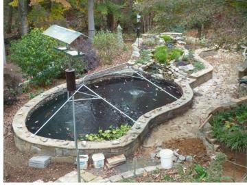
1/2" mesh bird netting is spread over two pyramids constructed of 3/4" Dia. Electrical conduit. (The bird feeder in the foreground is optional).
